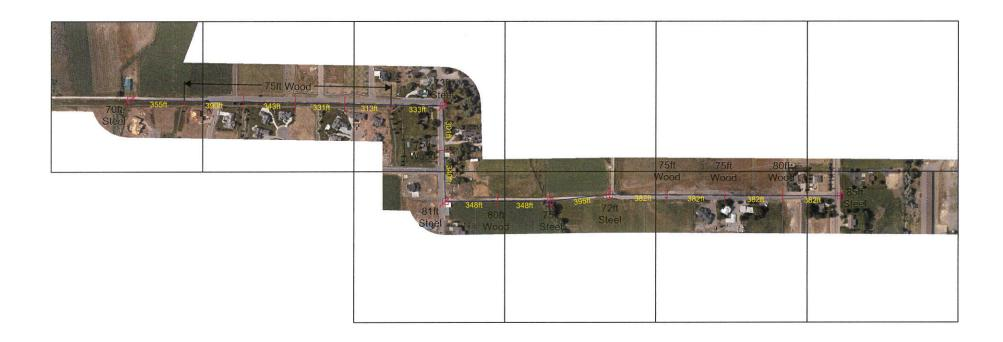
Reduced Pole Height Proposal Span Length: 185ft - 395ft 21 Total Structures Structure Height Above Ground: 65ft - 83ft
