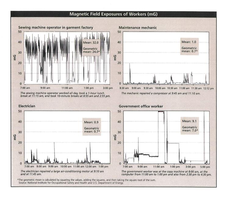
The tables below and on page 41 can give you a general idea about magnetic field levels for different jobs and around various kinds of electrical equipment. It is important to remember that EMF levels depend on the actual equipment used in
