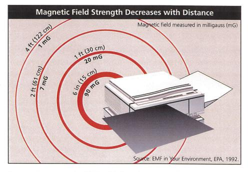
You cannot see a magnetic field, but this illustration represents how the strength of the magnetic field can diminish just 1–2 feet (30–61 centimeters) from the source. This magnetic field is a 60-Hz power-frequency field.
