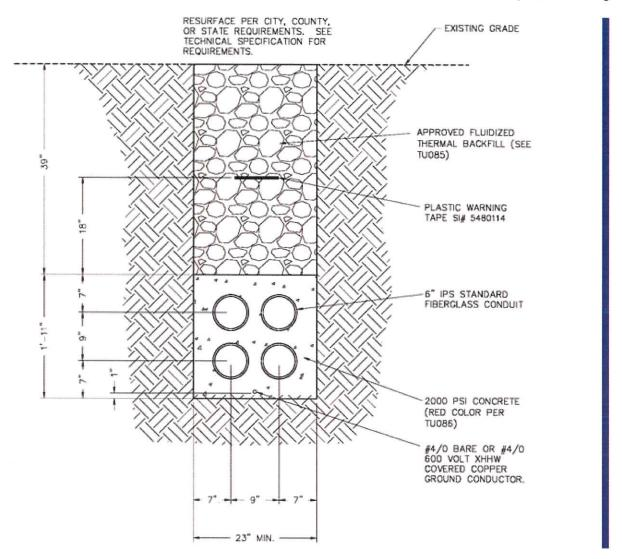
Figure I—Typical Single-Circuit Conduit Layout
