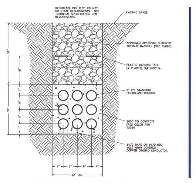
Figure 2—Typical Double-Circuit Conduit Layout
