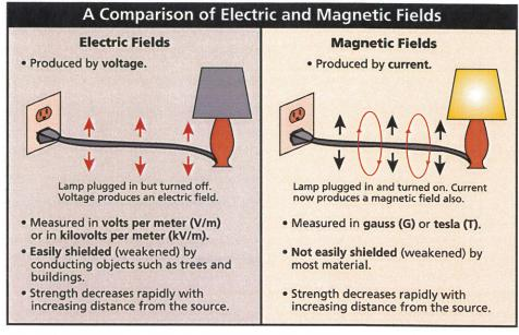
An appliance that is plugged in and therefore connected to a source of electricity has an electric field even when the appliance is turned off. To produce a magnetic field, the appliance must be plugged in and turned on so that the current is flowing.
